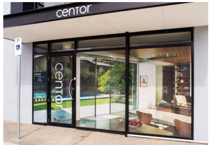
This is an example of a printed one way vision film. Note how the back layer is black to improve visibility from the inside out.
