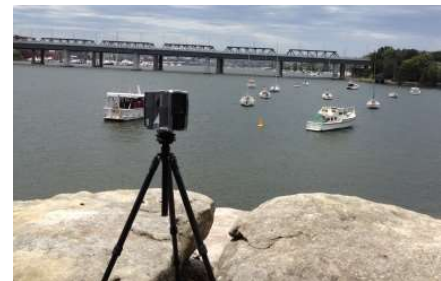
Terrestrial Surveying Scanner.
